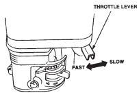
Figure 22. Throttle Lever
